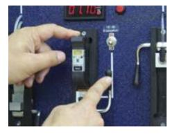
When the evacuation operation is completed, then remove the cartridge from the station, fliping the handle down
