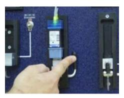
Flip the handle up to secure the cartridge
