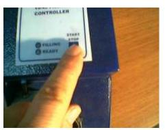
Push the Start/Stop button to start filling.Includingpressurizing machine will fill the cartridge in 2,5 minutes,when filling operation has completed place the cartridge into evacuation station and evacuate 2-3 seconds for priming.
