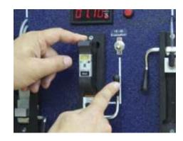
Place the cartridge to the 15/40/45 Evacuation Station and Flip the handle up to squeeze the cartridge
