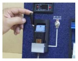
Be sure that the remaning ink is removed, and flip the handle down to take out the cartridge
