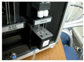
Needles will go down automaticly and filling process starts. When the cleaning process finished needles will go up.
