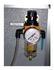
Pressure Regulator will be shipped you seperately , so first you will install it the place of it as shown above left side of the machine. Two screws are provided for the installation of pressure regulator , screw them together with the pressure regulator and fix it on the left side of the machine, connect the inlet tube to the pressure regulator and connect compressed air tube (6mm) to the pressure regulator as shown shown right.
