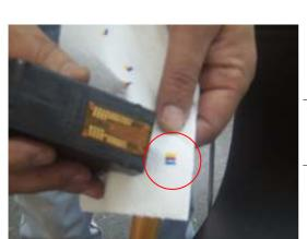
Test the cartridge by pushing on a clean tissue paper
