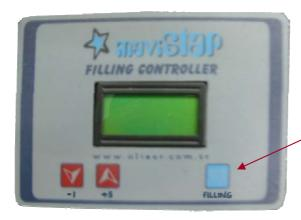
Push start/stop filling button to start cleaning process
