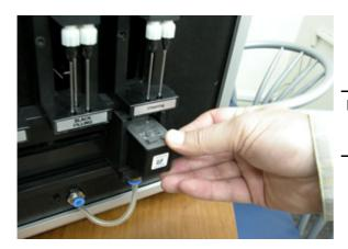
Insert cartridge into the cartridge holder
