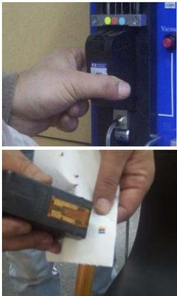
**Test the cartridge by pushing on a clean blotting towel**
