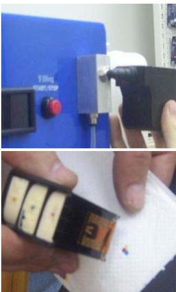
**Position the filled cartridge on vertical suction cup, Apply Low vacuum in one second pulses until distinct three color footprint is obtained on a clean blotting towel .**
