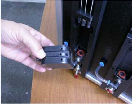
Be sure that fill hole plugs are removed!
