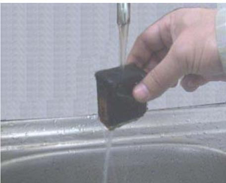
**Clean the cartridge bottom and the interior screens with pure distilled water.**
