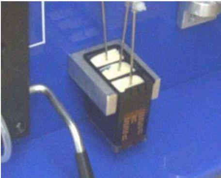
**Place the cartridge into the filling station**
