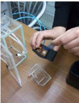
Take out the cartridge from the Filling Chamber
