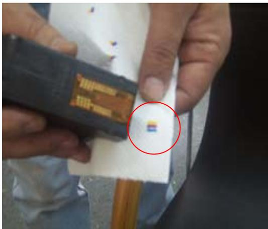
Test the cartridge by pushing on a clean tissue paper
