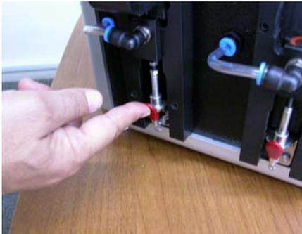
Lift the handle up and secure the cartridge, be sure that cartridge is tight.
