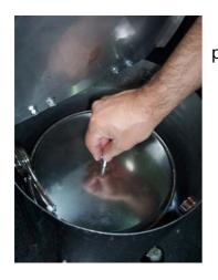
Secure the cartridges with plate as shown left.
