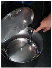
On/Off power switch placed on the right side of centrifuge, when the top cover is open, motor will stop automatically and start centrifuge when top cover closed.
