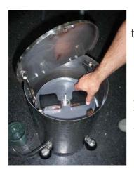
Place the cartridges as shown to get empty through fill hole plugs.
