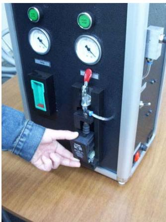
Insert the cartridge filling station as shown.
