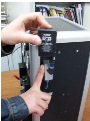
After filling completed, cartridges requires prime/balance, using the suching cup placed on the right side of the machine, such a few seconds ink from printhead
