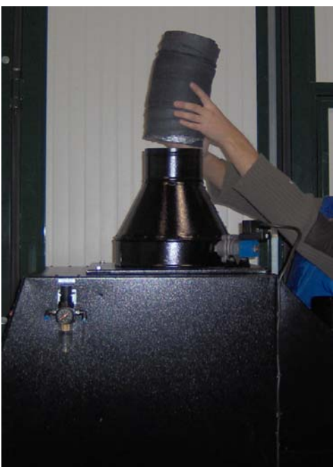
Place the accordion pass tube both side and fix them using pipe-clip
