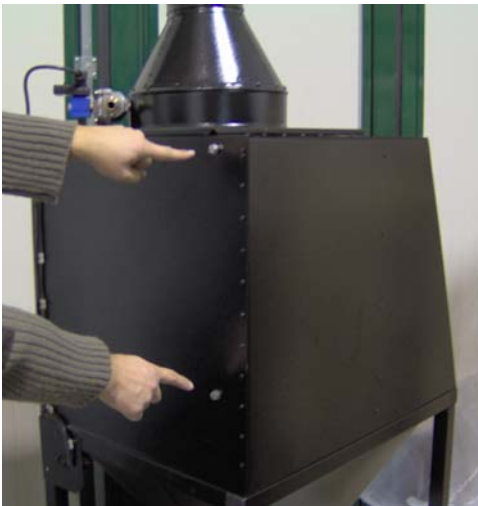
Take out the screws from rear of the machine and place the back unit using the screws
