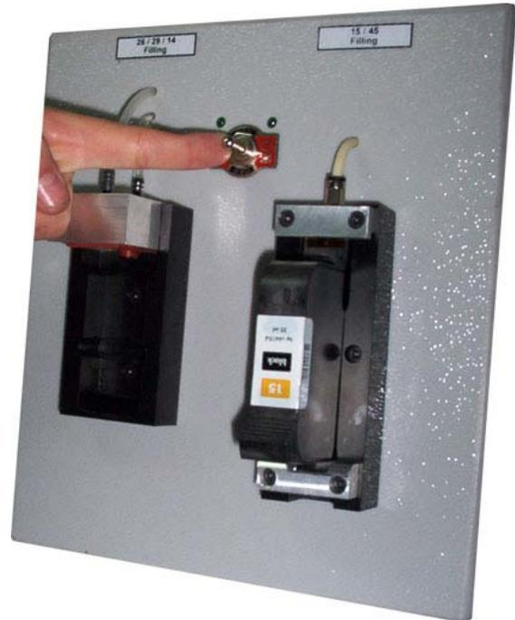
Flip the mode switch to 15/45 filling position.
