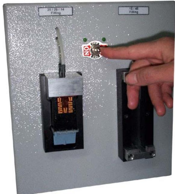
Flip the mode switch to 26/29/14 filling position.
