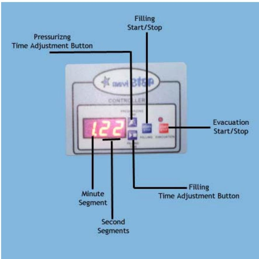
Adjust the timer around 2.20(2minutes,20seconds) and pressurizing 9seconds.
