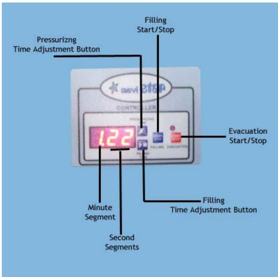
Adjust the timer around 2.20(2minutes,20seconds) and pressurizing 9seconds. Push to the filling button to start filling process.
