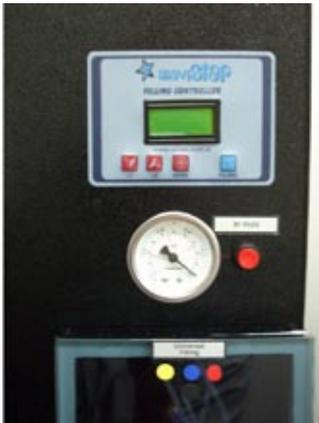
Adjust the ink volume. Close the cover of the filling chamber firmly and push to the start/stop button, it will start vacuuming and when reached to the correct vacuum level , automatically filling will start and stop after filling completed.
