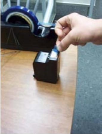
Seal the printhead of the cartridge using a blue tape.
