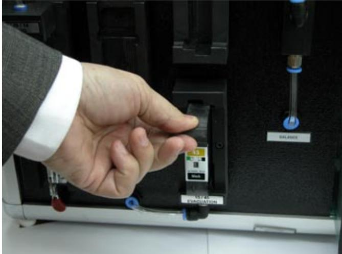
Place the cartridge in to the 15/45 evacuation station and switch on evacuation start/stop switch.
