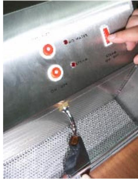
Please clean the cartridge print head using the steam generator. (Oliser sells TWO versions of Steam generators; one has a closed in housing, whereas the other is an open-environment unit)
