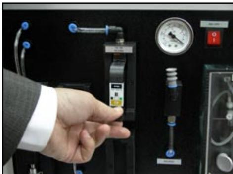
When the evacuation process is done , place the cartridge in to the 15/45 filling station.
