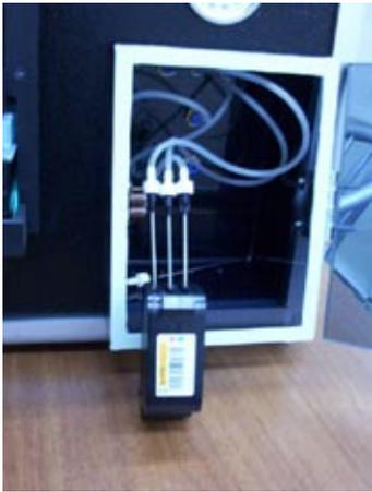
Insert the needles into the cartridge. Place the cartridge inside of the filling chamber.
