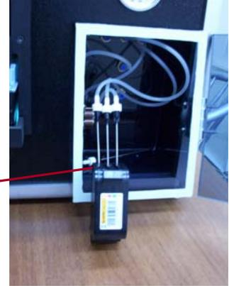
Insert the needles into the cartridge.
