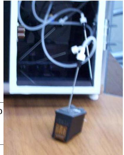
Adjust the ink volume. Close the cover of the filling chamber firmly and push to the start/stop button, it will start vacuuming and when reached to the correct vacuum level , automatically filling will start and stop after filling completed.
