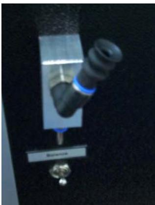
Take out the cartridge from the Filling Chamber, using the suction cup , do the priming operation , now cartridge is ready to print test.
